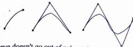
Curve doesn't go out of polygon boundary (Convex hull)
